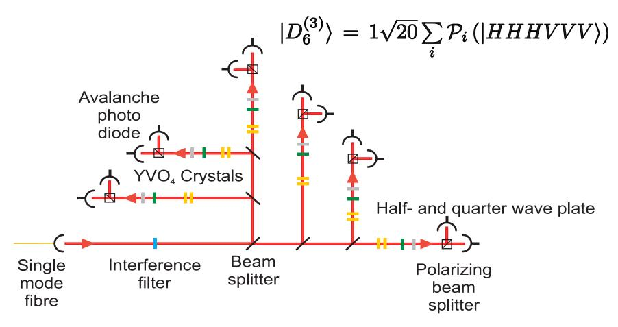
input state from the photon source is split up into spacial modes success rate of the setup is 1.3 % for six photons conditional detection scheme is applied
