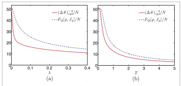
**Figure 2.** (a) The reciprocal of the parameter variance  $(\Delta\theta)_{\text{opt}}^2$  given in (21) and the quantum Fisher information for the ground states of the spin-squeezing Hamiltonian (27) as a function of  $\lambda$  for N = 100 particles. (b) The same quantities are shown for the thermal states (29) as a function of T.
