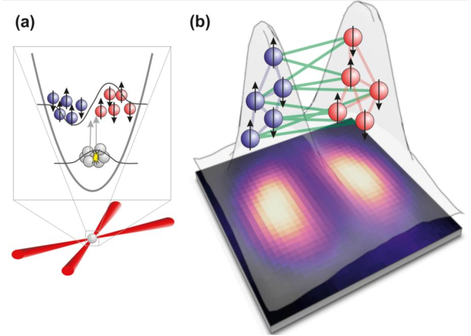
Pictorial representation of the experiment: entanglement is achieved between two clouds of atoms starting from a single Bose-Einstein condensate. Drawing by: lagoba Apellaniz, UPV/EHU
