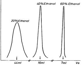
Fig. 3. Elution pattern obtained when  $[1^{25}I]PSTME$  was chromatographed using ethanol-water binary eluent of different concentrations.
