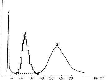
Fig. 2. Elution pattern obtained when the labelling mixture from the chloramine-T procedure and tritiumlabelled PSTME were chromatographed. Peaks: 1 =free radioiodine; 2 =tritium-labelled PSTME; 3 =<sup>125</sup>I-labelled PSTME.
